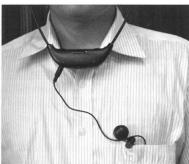
To use the receiver as a wired listener plug one end of the stereo patch lead into the LINE IN or MIC IN socket on the receiver and connect the other end to an audio source such as PC, Radio, MP3, etc. Ensure the volume on the receiver is set to off, then switch on the receiver and adjust the volume and tone to your required levels.
